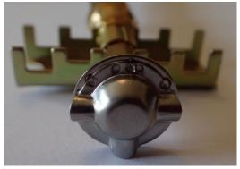
Step 4. Lay the pilot assembly into the bracket. **Note the direction of the pilot jets.**
