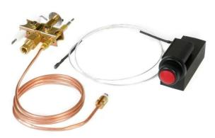
You may find it easier to replace the pilot assembly with the pilot cage removed. Straighten the cage legs to remove it. Disconnect the lead from the white ceramic electrode, under the pilot. Disconnect the copper thermocouple from the back of the valve by unscrewing the small brass split nut. **Do not loosen or remove the large silver nut** that forms part of the main gas valve.
