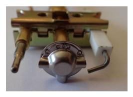
Carefully uncoil the copper thermocouple and slip the small brass split nut over the flattened part at one end. Push into the back of the gas valve and tighten the split nut. Ensure the copper lead is not kinked or bent sharply, as this will render it inoperative.
