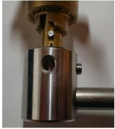
To let gas through to the pilot, turn the lever so the handle points to the spark position, at 2 o'clock on the control box, and push in. Note the pin on the shaft engages with the slot in the valve body. The handle and valve should look like this:
