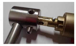
With the handle pointing to the black dot, at 3 o'clock on the control box, this is the off position. The handle and valve should be orientated like this:
